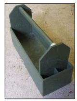
"The ends, sides and base of the tool carry body is made from a 17cm wide strip of 6mm flake board, but think ply would have been better.
